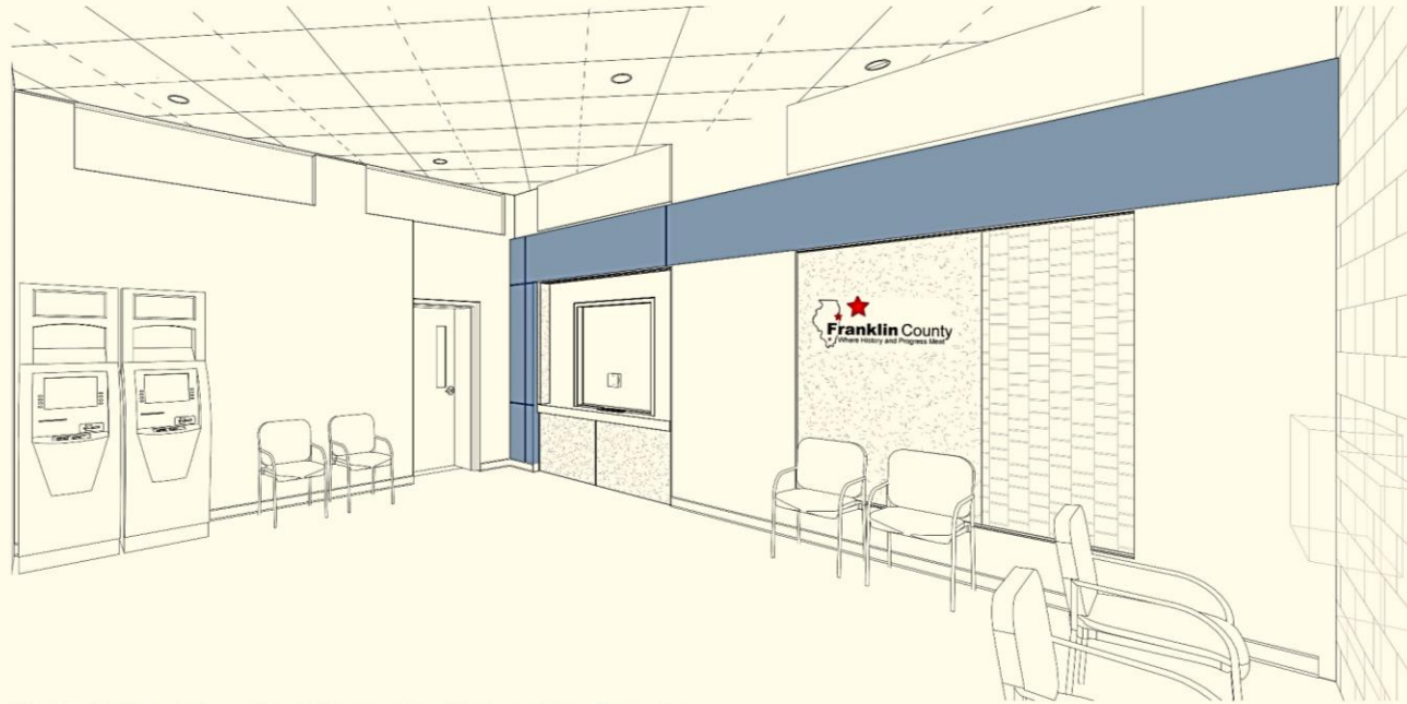
3D view Service window with portal surround and feature niche with signage
